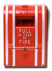
All non-coded statins are designed for either flush or surface mounting. For flush mounting a 4 inch standard North American square box with single gang plaster cover should be used. For surface mounting the 270 Series or 270P Series, use P-027193 Cast Box, P-039250 Steel Box, or Cat. No. 1291 Housing for weatherproof enclosure.
